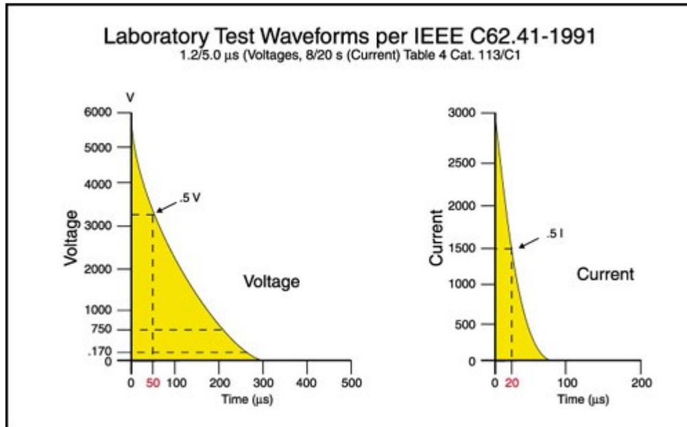
For short duration testing we would apply up to a 6kV, 1.2/50 voltage wave form into an open circuit with the TVSS device across it. Here, the voltage reaches 90% of its peak in 1.2 μs and then decays to 50% of its value in 50 μs.
