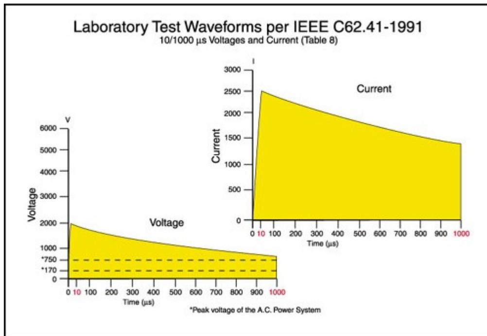
For long duration testing, the waveform will have a peak value of 2kV with a rise time of 10 μs and a duration 1000 μs. The current waveform has a peak of 2.5kA with the same rise and duration times (10/1000 μs)
