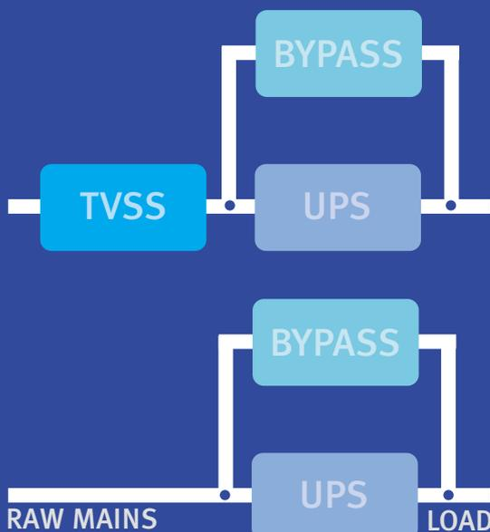
← Load connected to lightning and transient path when the UPS fails or is overloaded
