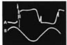
There is a limit to the dynamic range afforded by most designs but all CVT's exhibit the ability to provide a stable output voltage curve from a varying source. Although usually specified over a  $\pm 15\%$  range the CVT does not just 'stop' outside this voltage range.
