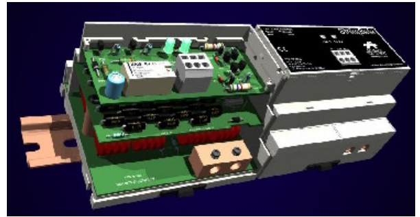
Cutaway of Din rail mount TDC 200kA showing multi stage matrix
