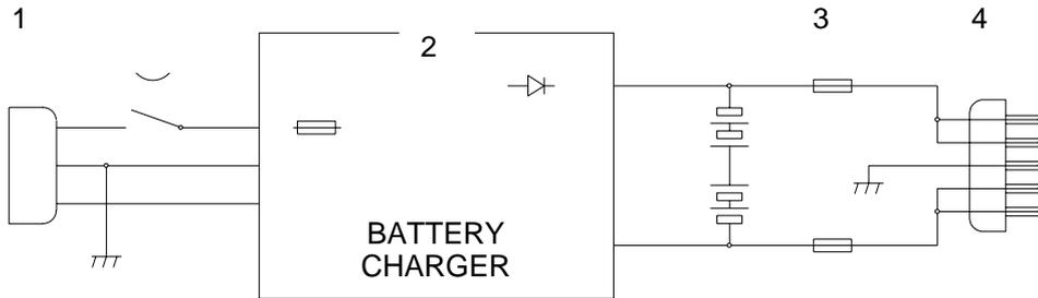
Diagram 1: PRS with built-in batteries and charger
